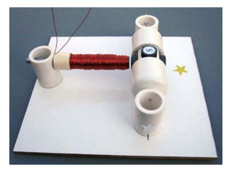
13. For Kit #5 attach the self-sticking felt pad to the reed switch stand as shown on the left picture below. The picture on the right side shows how to attach the felt pad to the universal reed switch/Hall effect switch stand for Kit #8. This soft pad decreases the reed switch vibration thus decreasing the sound it generates.
