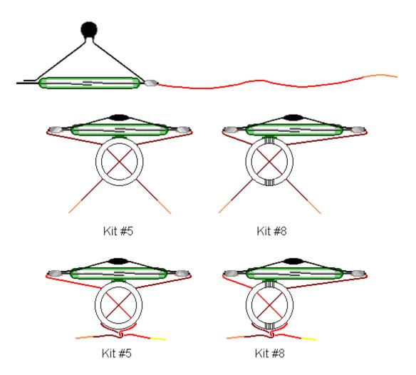
16. Use rubber band to prevent the reed switch from moving.
