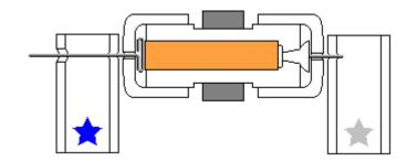
8. Glue the stand with the silver star to the board. Try to cover the corresponding star completely. Align the marks on the stand with the line on the board as shown below. Note that the star's position and the marks are approximate, sometimes you need to move the stands slightly to achieve the lowest friction. Keep in mind that super glue bonds instantly, so try to be as accurate as possible in these procedures.
