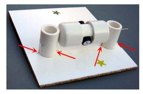
9. Insert the rotor into the stand marked with the blue star. Glue it to the board the same way as the first stand. Leave a gap of about 1/16" (1/32", or 0.8mm on each side) between the rotor and the stands. Test again to see if the rotor spins freely. At this time, or later, you may take the rubber plug and fix it as shown below. You can glue different things to the outer flat surface of the plug. Try to be accurate, redo this step if necessary.
