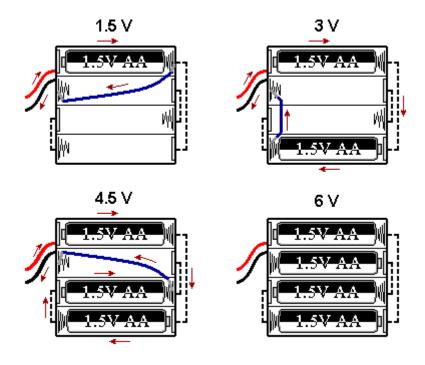
Insert bare ends of the jumper wire between the spring and plastic case to make a good contact and hold them in place. This is how the jumper wire is actually used for 1.5 Volts experiments (one end is disconnected and may serve as on/off switch):
