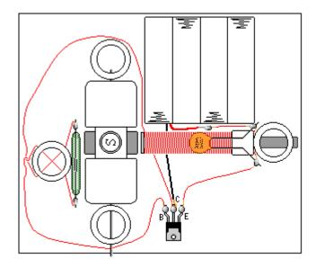
21. You may connect a capacitor as shown in the diagram above. Do not forget to remove the insulation from the magnet wire before soldering. It is not a required part for the motor to work, but it may prolong the life of the reed switch. However using the ZNR as shown in step 15 usually provides better results.
