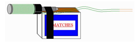
4. Using the duct tape attach the matchbox to the board as shown below.
