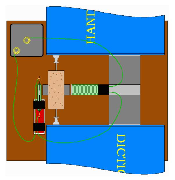
11. Before connecting everything together connect both wires from the electromagnet to the battery. If the electromagnet doesn't repel the permanent magnets away, switch the wires. When it repels, disconnect one wire and connect it to the reed switch. Connect the other end of the reed switch to the battery as shown on the picture above.
