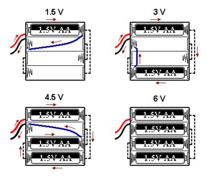
Insert bare ends of the jumper wire between the spring and plastic case to make a good contact and hold them in place.
