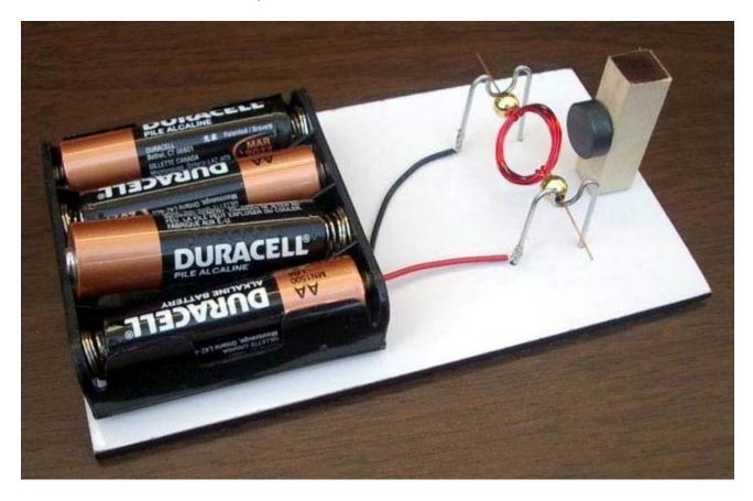
This is the motor with two magnets on the sides.
