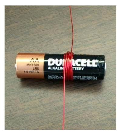
2. Carefully remove the battery and wrap the ends around the coil 2-3 times to hold the coil together with both ends extending perpendicular to the coil as shown below. The ends should be aligned in a straight line to form a good axle. This step requires a lot of accuracy because the balance of the coil is extremely important.
