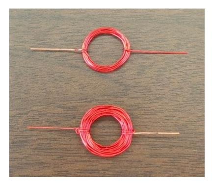
3. Strip off the insulation completely at one end and only half of it at the other. This step is very important, try to be very accurate.
