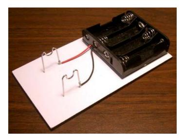
6. The battery holder and a jumper wire included in this kit allow you to experiment with 4 different voltages: 1.5, 3, 4.5, and 6 Volts. To understand how the jumper wire works let's take a look at the connections inside the battery holder:
