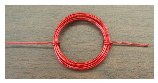
The kit contains enough wire to experiment with the coils of different size (10 and 30 windings shown).
