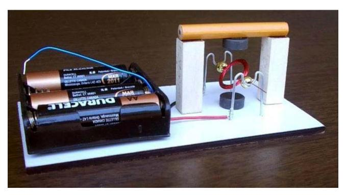
You may have the magnets placed sideways as shown in the pictures below. However, when you strip half of the insulation as explained in step 3 you should lay the coil flat on the table or hold it so it is in a horizontal position.
