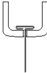
2. Insert the rotor core into the same cap as shown below. Apply some pressure to push the rotor core approximately 1/2" (10-12mm) into the cap.
