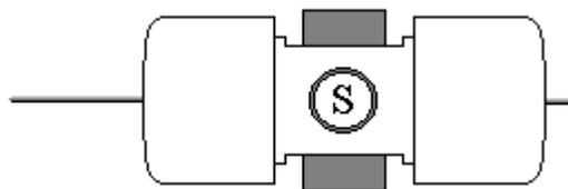
7. Insert the rotor into the stands marked with blue and silver stars as shown below. Hold the stands and test to see if rotor spins freely. Make final adjustments to the T-pin if necessary.
