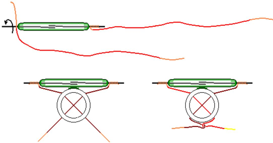
15. If you want to experiment with higher voltages (up to 15 Volts) or make much more reliable motor you may add a ZNR. The ZNR is a small electronic part that absorbs the spark inside the reed switch. The ZNR is not required for the motor to work. Skip this step if you are not adding ZNR at this time.
