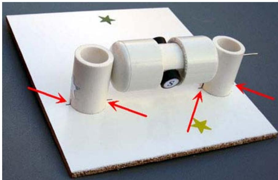
9. Insert the rotor into the stand marked with the blue star. Glue it to the board the same way as the first stand. Leave a gap of about 1/16" (1/32", or 0.8mm on each side) between the rotor and the stands. Test again to see if the rotor spins freely. At this time, or later, you may take the rubber plug and fix it as shown below. You can glue different things to the outer flat surface of the plug. Try to be accurate, redo this step if necessary.
