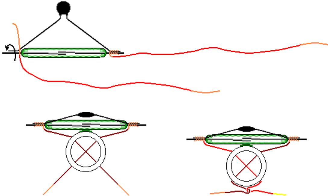
16. Use rubber band to prevent the reed switch from moving.
