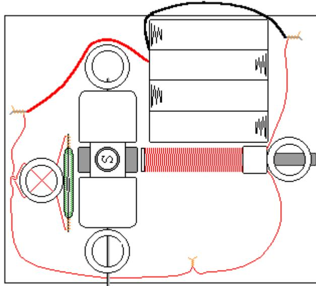
Start with 1.5V. If the motor does not work, increase the voltage to 3V. If it doesn't help, ensure that the rotor rotates freely and check all the connections – it is important to clean the insulation thoroughly. Make sure the batteries are fresh and connected properly. If the motor still does not work – check Troubleshooting section of our web site.
