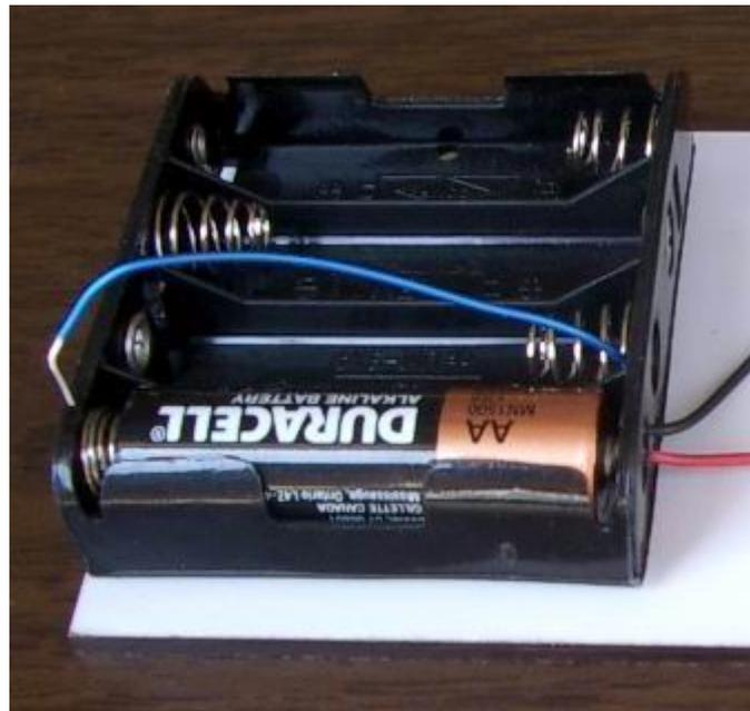
19. Before connecting everything together connect both wires from the electromagnet to the battery. If the electromagnet doesn't repel the permanent magnets away, switch the wires. When it repels, disconnect one wire and connect it to the reed switch. Connect the other end of the reed switch to the battery. You may tape the wires to the board using scotch tape. The wiring diagram for kits #3 and #4 is shown below:
