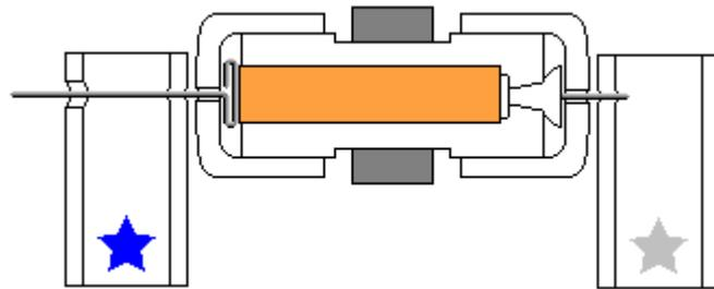
8. Glue the stand with the silver star to the board. Try to cover the corresponding star completely. Align the marks on the stand with the line on the board as shown below. Note that the star's position and the marks are approximate, sometimes you need to move the stands slightly to achieve the lowest friction. Keep in mind that super glue bonds instantly, so try to be as accurate as possible in these procedures.
