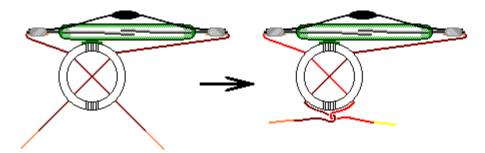
21. Bend the leads of the Hall effect switch as shown below. If your kit includes 1 large piece of hook-up wire, cut 4 pieces with the length of 8-9" (20-23cm) each. Strip about 3/8" (10mm) of insulation on each end of these wire pieces using a sharp knife. Solder three wire pieces to the Hall effect switch.
