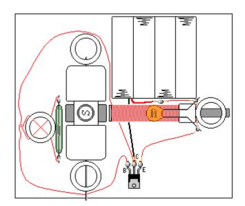
This is the wiring diagram for the reed switch motor with transistor:
