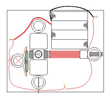
This is the wiring diagram for the reed switch motor:
