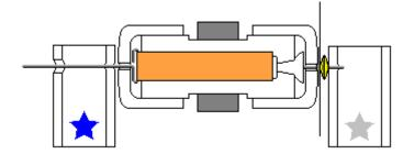
9. Glue the stand with the silver star to the board. Try to cover the corresponding star completely. Align the marks on the stand with the line on the board as shown below. Note that the star's position and the marks are approximate, sometimes you need to move the stands slightly to achieve the lowest friction. Keep in mind that super glue bonds instantly, so try to be as accurate as possible in these procedures.
