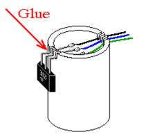
24. Glue the universal stand to the board. The Hall effect switch and reed switch should be located in front of the magnets at the closest distance. Check the rotation of the rotor to make sure that the magnets do not hit any of the switches.
