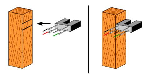
17. Glue the optointerrupter stand to the board as shown in the picture. If you rotate the rotor, the disk blades should be in the middle of the slot as deep as possible without hitting the optointerrupter. Wait for the glue to dry. Hold the middle part of the rotor and rotate the cap that has the disk attached until one of the blades is inside the slot. You will need to experiment with it later to find the best position of the disk to provide a good start and the best speed.
