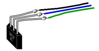
23. Insert the Hall effect switch into the universal stand. For simplicity it is shown without the reed switch, which will be located below the Hall effect switch. Make sure that the leads of the Hall effect IC do not touch each other. You may add a drop of glue to keep the IC and wires in place. Glue only the leads, do not glue IC case to the stand.
