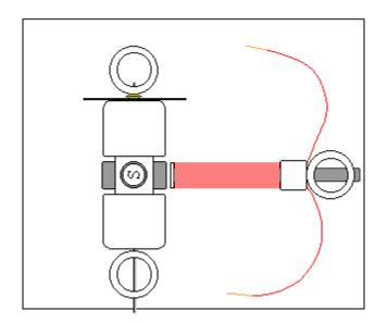
14. Locate the optointerrupter pins as shown on the following picture. It is very important to identify all four pins properly. Wrong connection in the motor will destroy the optointerrupter.
