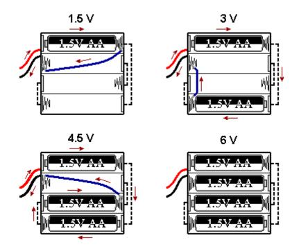
Insert bare ends of the jumper wire between the spring and plastic case to make a good contact and hold them in place. This is how the jumper wire is actually used for 3 Volts experiments (one end is disconnected and may serve as on/off switch):
