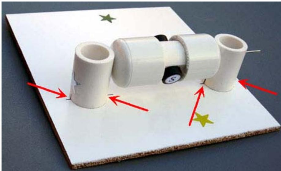
10. Insert the rotor into the stand marked with the blue star. Glue it to the board the same way as the first stand. Leave a gap of about 1/16" (1/32", or 0.8mm on each side) between the rotor and the stands. Test again to see if the rotor spins freely. At this time, or later, you may take the rubber plug and fix it as shown below. You can glue different things to the outer flat surface of the plug. Try to be accurate, redo this step if necessary.
