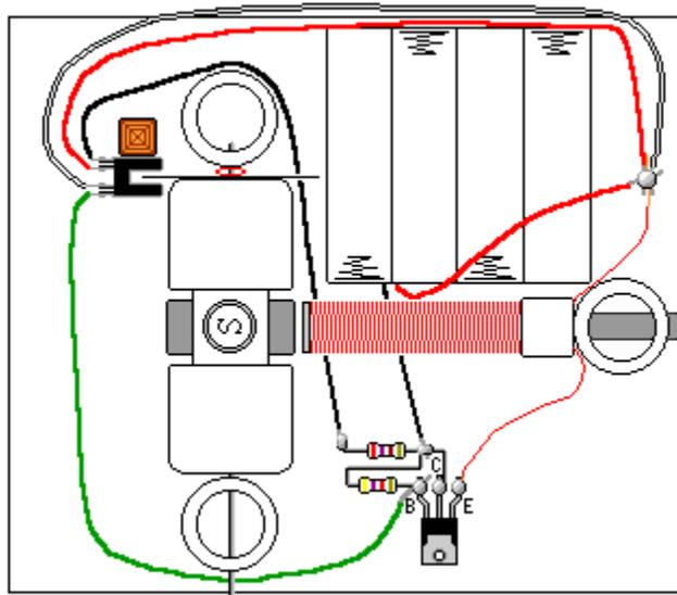
Check your connections carefully! Even a brief connection of the optointerrupter wires directly to the battery may destroy it.
