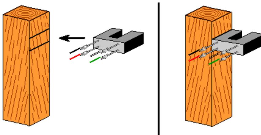
17. Glue the optointerrupter stand to the board as shown in the picture. If you rotate the rotor, the disk blades should be in the middle of the slot as deep as possible without hitting the optointerrupter. Wait for the glue to dry. Hold the middle part of the rotor and rotate the cap that has the disk attached until one of the blades is inside the slot. You will need to experiment with it later to find the best position of the disk to provide a good start and the best speed.
