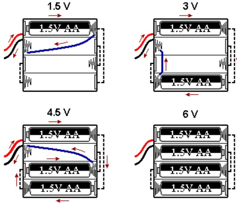
Insert bare ends of the jumper wire between the spring and plastic case to make a good contact and hold them in place. This is how the jumper wire is actually used for 3 Volts experiments (one end is disconnected and may serve as on/off switch):
